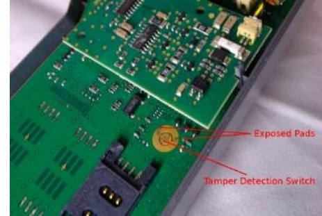
Switches on a PCB for detecting tamper [1]
