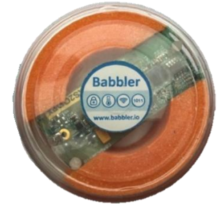
Digital seal for detecting openings of cargo containers through vibration sensors [2]
