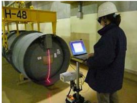
Laser based inspection of storage container [6]
