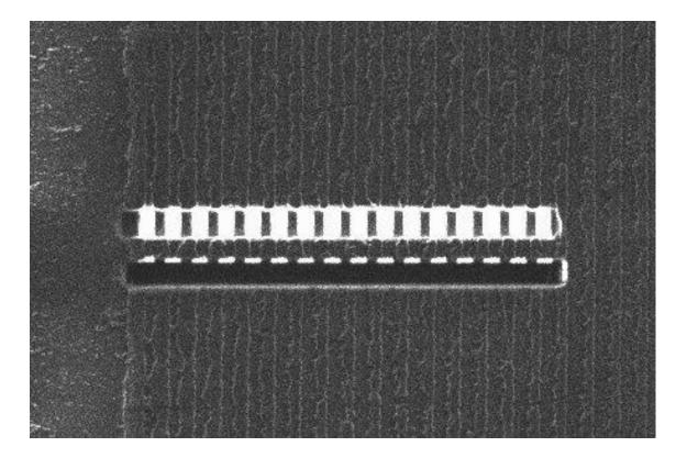
Expose the circuit lines of the second column of contacts
