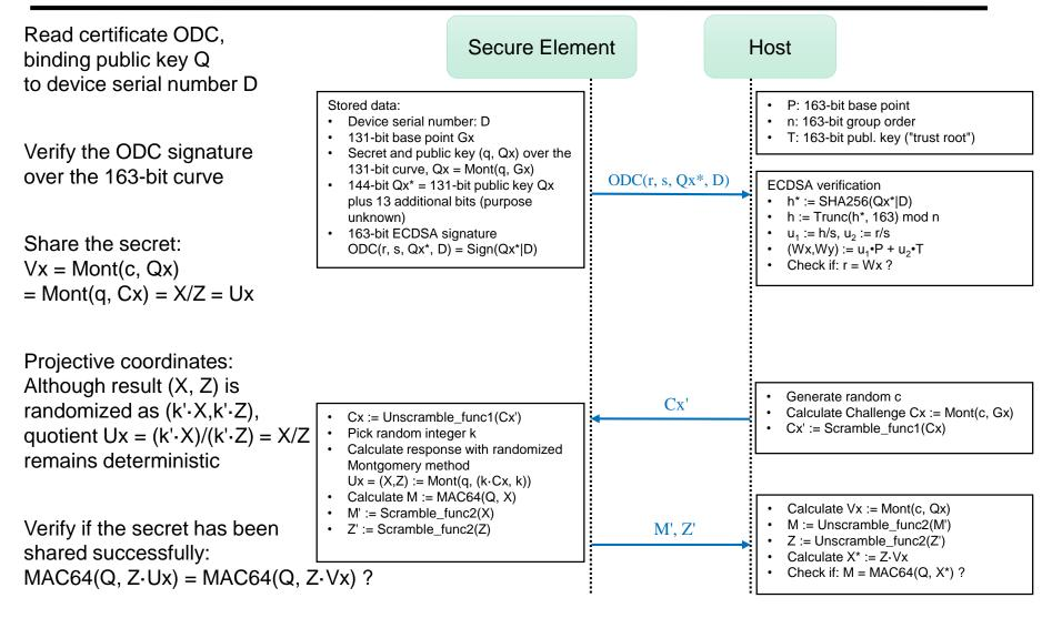
Great dot •: scalar muplication over EC ((Wx,Wy) :=  $u_1 \cdot P + u_2 \cdot T$ ), both coordinates x, y get involved. Mont(s, Px): scalar muplication over EC with Montgomery method, only coordinate x gets involved. Small dot ·: muplication over GF(2<sup>131</sup>)/f(x), f(x) = x<sup>131</sup> + x<sup>8</sup> + x<sup>3</sup> + x<sup>2</sup> + 1
